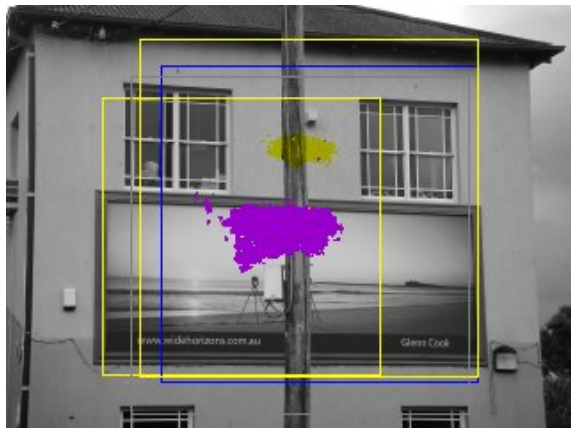
Figure 6: Results of the method depend on the image resolution. With higher resolution the cloud of candidate box center points shrinks.
